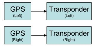
There are two GPS receivers (MMR or GNSSU). One GPS receiver provides data to the LEFT side transponder, and the other provides data to the RIGHT side transponder.
